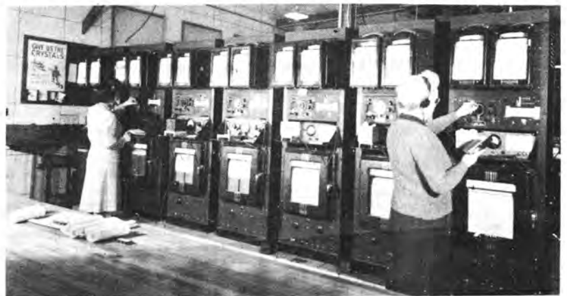
TESTING PRE-PRODUCTION SAMPLES OF CRYSTALS PRODUCED FOR SIGNAL CORPS.
